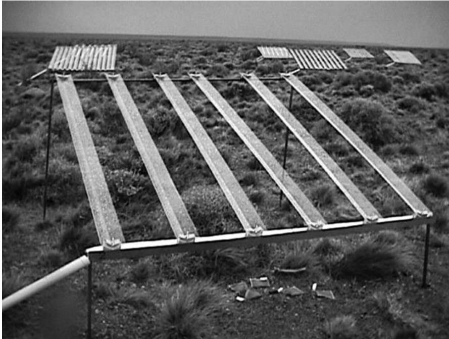
PLATE 1. Rainout shelters in the Patagonian steppe employed to intercept different amounts of incoming rainfall, simulating droughts of differing intensity. Photo Credit: L. Yahdjian.
